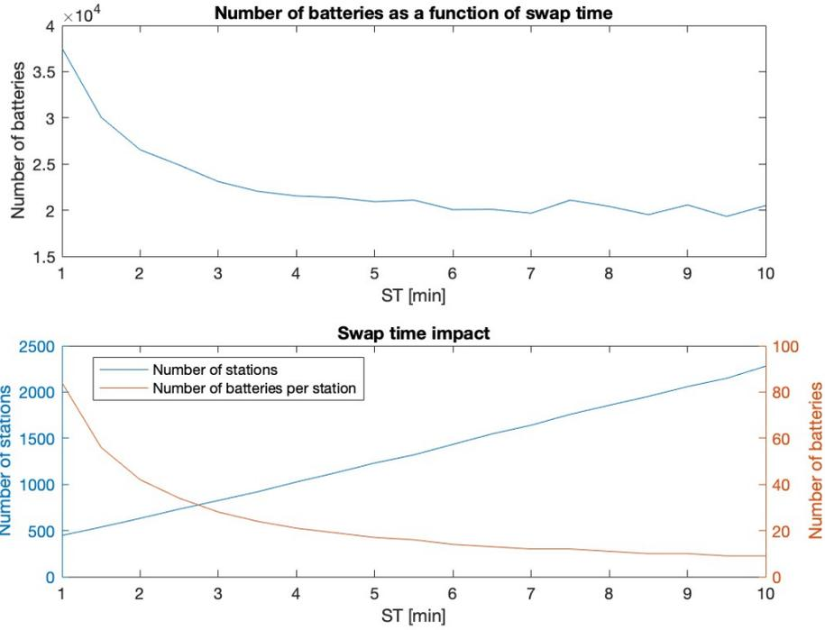
Figure 33: Number of batteries, ST.
