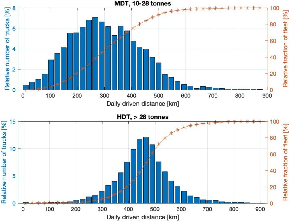
Figure 6: Trip distances, medium- and heavy-duty trucks [6].
