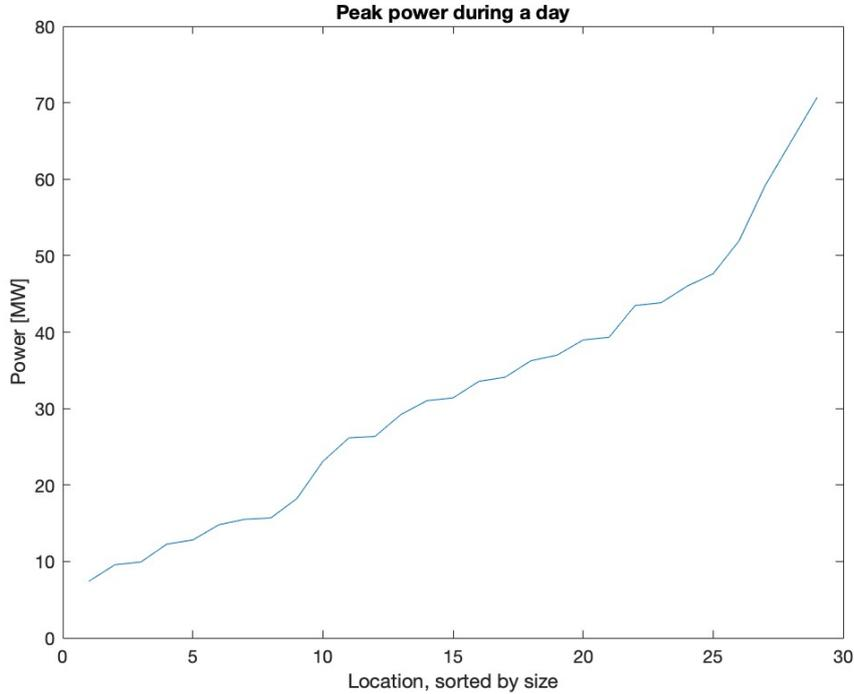
Figure 22: Peak power levels per location in a day, sorted by size.
