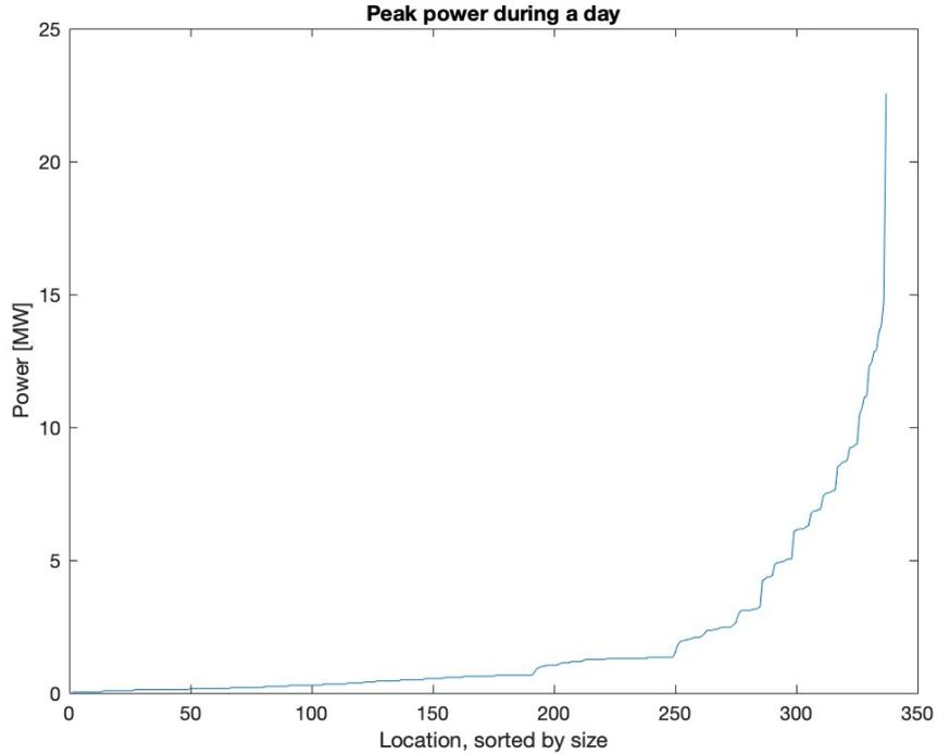
Figure 15: Peak power levels per location in a day, sorted by size.
