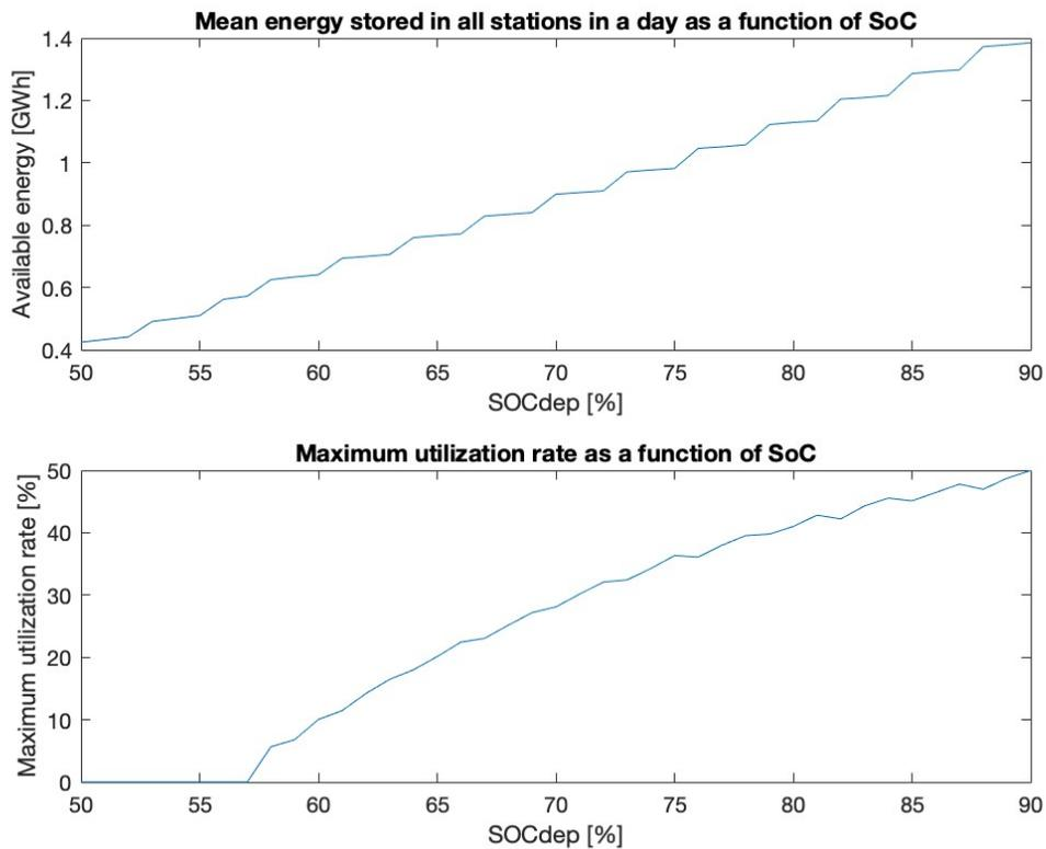
Figure 25: Available energy and utilization rate, SOCdep.
