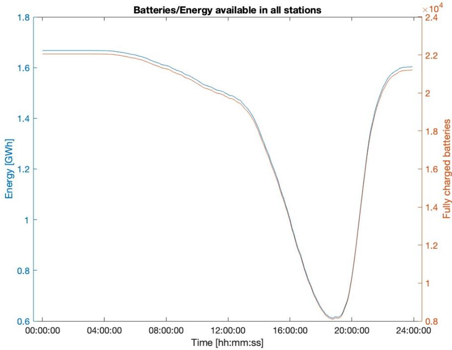
Figure 13: Fully charged batteries stored in BSSs.
