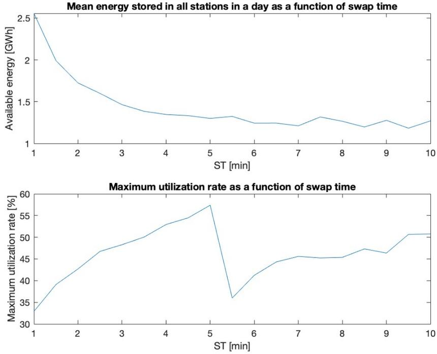
Figure 36: Available energy and utilization rate, ST.
