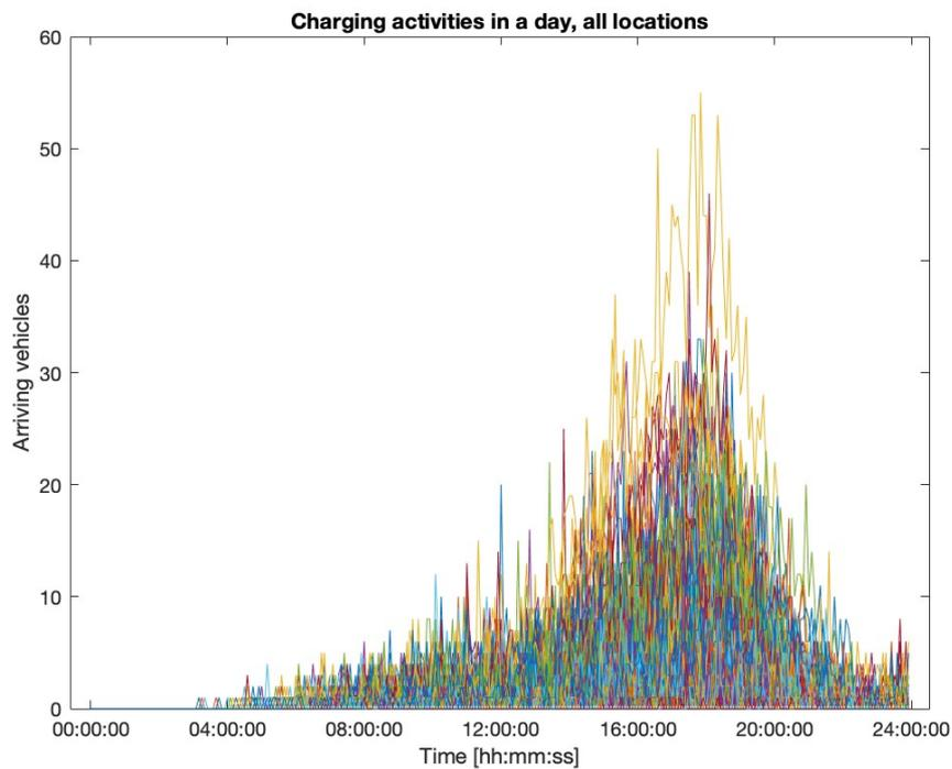
Figure 9: Aggregated charging needs at all locations during a day.
