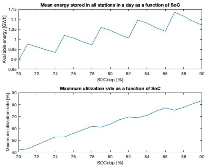
Figure 39: Available energy and utilization rate, SOCdep.
