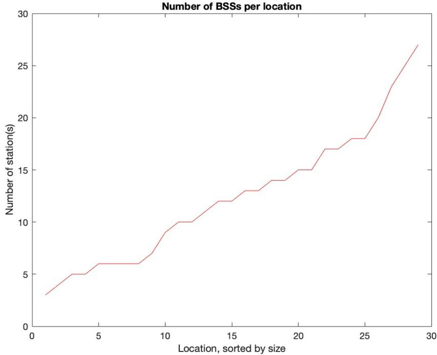
Figure 19: Number of BSSs per location to satisfy the truck queue requirement, sorted by size.
