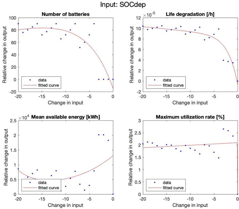
Figure 37: Relative change in output (absolute values) to input, SOCdep.
