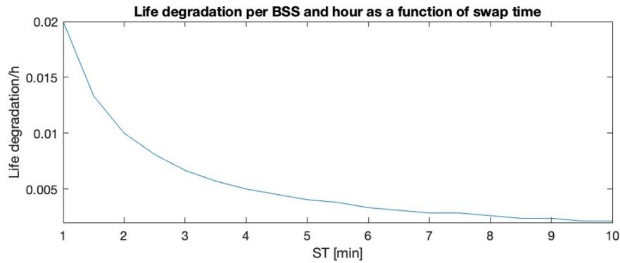
Figure 35: Life degradation, ST.
