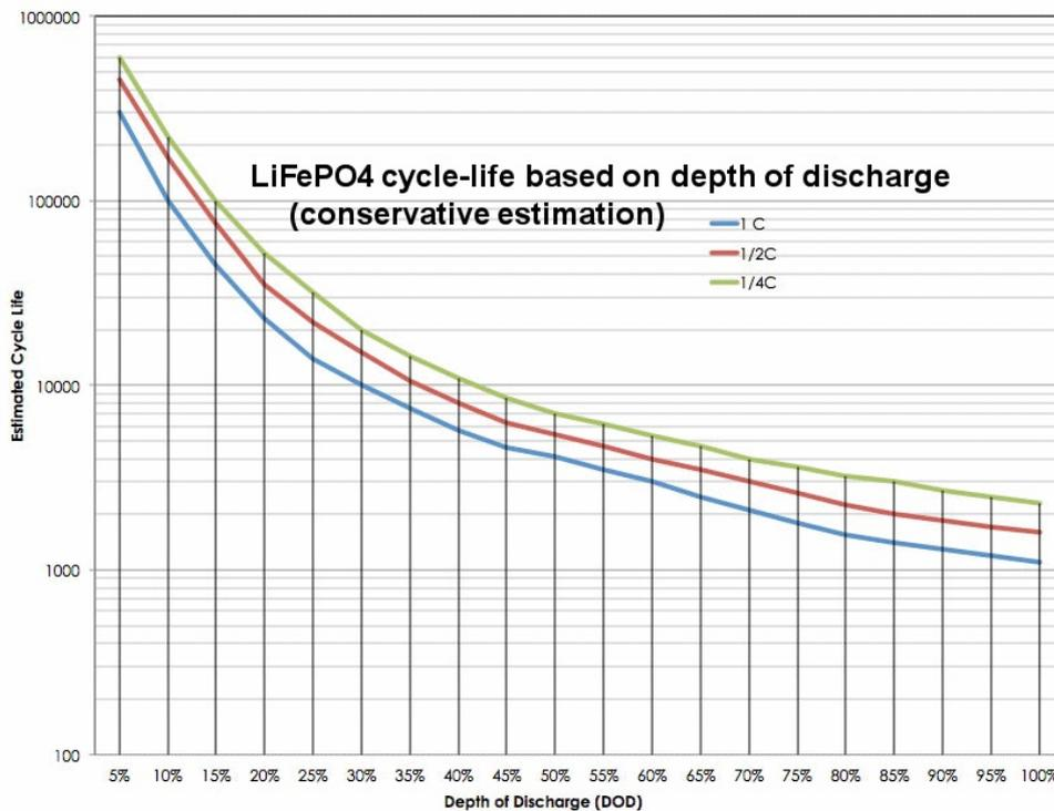
Figure 8: Estimations of the life-cycle of a LiFePO<sub>4</sub> battery based on the depth of discharge and discharge rate [8].
